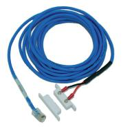
The magnetic door contact is a security feature for door and side panel monitoring. With the magnetic door contact it is possible to monitor unauthorized opening of doors as well as side panels. The contact is powered from the main unit. The extension is performed using a standard CAT 5/6 network cable and an RJ45-RJ45 coupler (category 5e) RMS-I-CON. The maximum length of the extension cable is 300 m.
