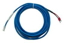
The dry contact sensor is used to connect external devices, such as security or fire systems, or any application that requires control by the unit. When used as an output, it can supply up to 20 mA. The input power supply range is 0 to 5 V. The contact is powered from the main unit. The extension is performed using a standard CAT5/6 network cable and an RJ45-RJ45 coupler RMS-I-CON. The maximum length of the extension cable is 300 m.
