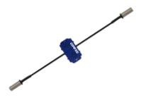
Thermal map sensors are ideal for complete environment monitoring in the racks. By using this device it is possible to determine hotspots and adjust the installation of IT hardware in the rack or regulate the output of the cooling unit. Pre-wired sensors on cable string monitor rack in 3 levels.
