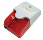
The sensor detects the presence or absence of flowing air inside the racks. The sensor works on the principle of differential measurement, which compares the resistance of the external and internal thermistor. This device can be connected to an alarm response and can be extended up to 30 m using a LAN CAT 5/6 cable.
