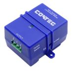
Mini Relay box with optional controlled power output can be plugged into RAMOS Plus or Optimax main monitoring units. This device can drive the larger relay with optional low current output. Equipment with a relay that needs to be switched based on sensor input, this adapter will switch contacts or output 200 mA—5 V DC based on a sensor's status.
