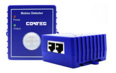
Motion detector with 60° detection angle and 3 m detection distance; used for securing rooms or buildings and sending alerts in case of intrusion into the monitored zone. It has a LED indication of the device status. Up to 10 motion sensors can be chain linked to a single smart port. Maximum total LANCAT 5/6 cable length for 10 sensors is 46 m. Maximum cable length between individual sensors should be less than 6 m. Maximum connectable cable length for a single sensor is 300 m.
