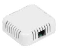
It measures the temperature, humidity and CO2 content of the air.
